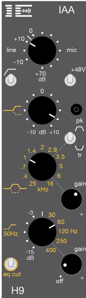
The GAIN knob adjusts the gain of the preamplifier. In the first three positions, it is in line input mode, which bypasses the mic input transformer and engages a pad. Line mode also disconnects phantom power from the input. In the final seven modes, the net gain is adjusted to the amount indicated. A pad is automatically engaged in the first two positions.
